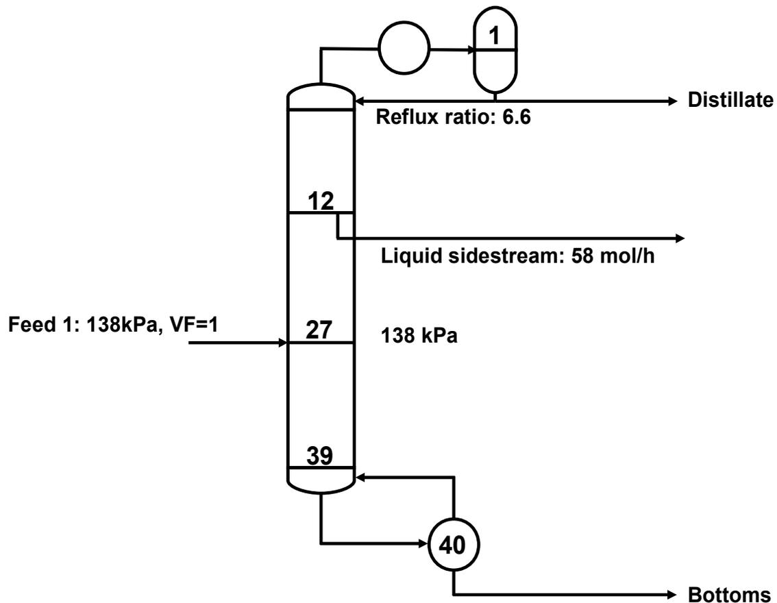
This column is used to recover a paraffin cut from straight kerosene. The feed is a mixture of “hypothetical” compounds with the following flowrates:
